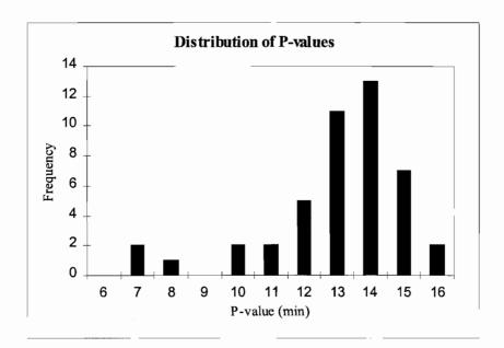
Figure 8: Distribution of pasteurisation values for the 325 kg batch of 20 mm apricot fool yogfruit, calculated with  $D_{85} = 6.95$  minutes. Sample size was 45.
