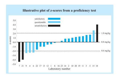
The figure shows the z-scores obtained by several laboratories. z-scores between -2 and +2 indicate a satisfactory performance. Z-scores between -3 and -2 or between +2 and +3 indicate a questionable result. Z-scores outside the range -3 to +3 indicate an unsatisfactory result. Where a laboratory obtains a 'questionable' or 'unsatisfactory' result, it should investigate the cause.
