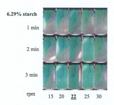
Table 4: Optimised rotation speeds for mixing in the product at different temperatures.
