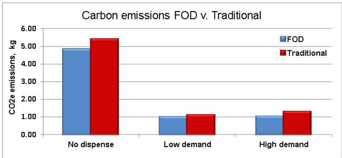
Figure 1 CO<sub>2</sub>e emissions for FOD and traditional dispense systems and the 3 different dispense scenarios (24hr no dispense, low demand: 20 pints in 1hr + 2hrs recovery, high demand: 60 pints in 1hr + 2hrs recovery)
