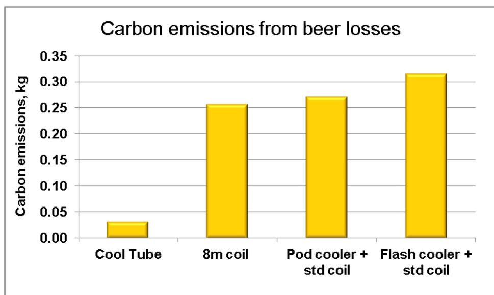
Figure 2 Difference in carbon emissions between beer held in CoolTube, 8m cooling coil, pod cooler + standard cooling coil or Flash cooler + standard cooling coil
