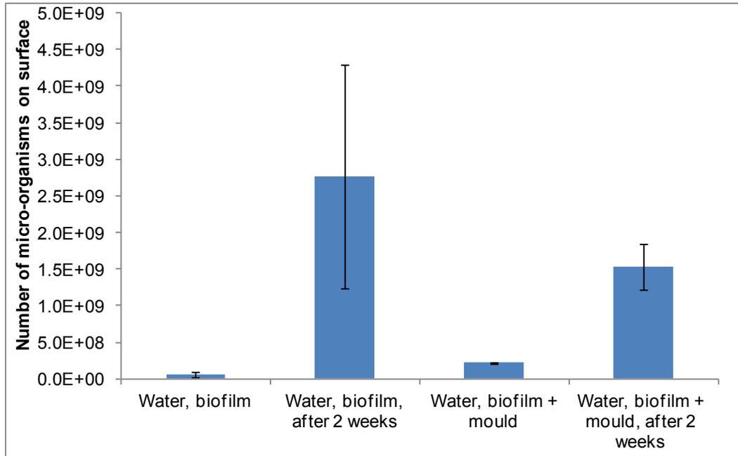
**Figure 4:** Level of contamination on stainless steel surfaces contaminated either with biofilm or biofilm containing mould and cleaned with 80°C water. One set of surface samples was re-incubated for 2 weeks following the cleaning procedure.
