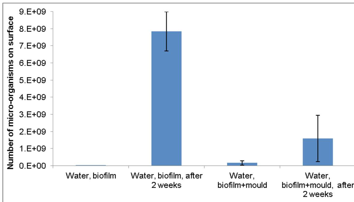
**Figure 2:** Level of contamination on tile surfaces contaminated either with biofilm or biofilm containing mould and cleaned with 80°C water. One set of surface samples was re-incubated for 2 weeks following the cleaning procedure.
