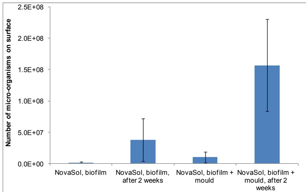
**Figure 5:** Level of contamination on stainless steel surfaces contaminated either with biofilm or biofilm containing mould and cleaned with 10% w/w NovaSol. One set of surface samples was re-incubated for 2 weeks following the cleaning procedure.
