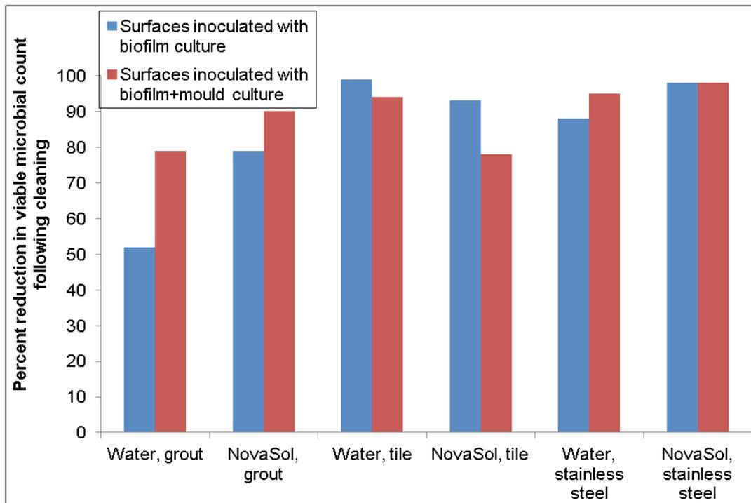
**Figure 1:** Percentage reduction in viable micro-organisms present on the different surfaces contaminated with biofilm culture with or without a common mould and treated with either water at 80°C or NovaSol at 10% w/w
