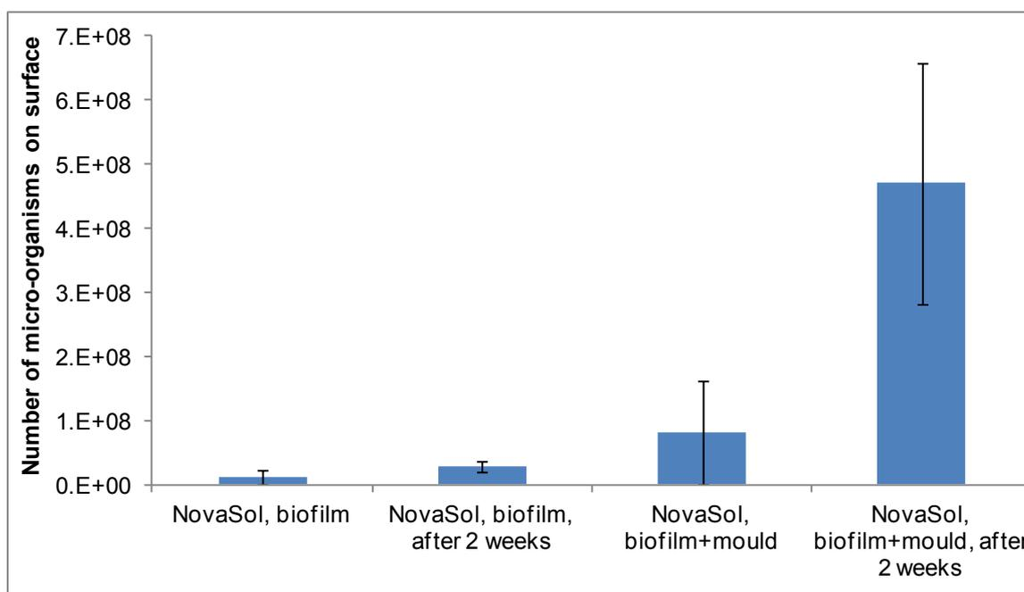
**Figure 3:** Level of contamination on tile surfaces contaminated either with biofilm or biofilm containing mould and cleaned with 10% w/w NovaSol. One set of surface samples was re-incubated for 2 weeks following the cleaning procedure.
