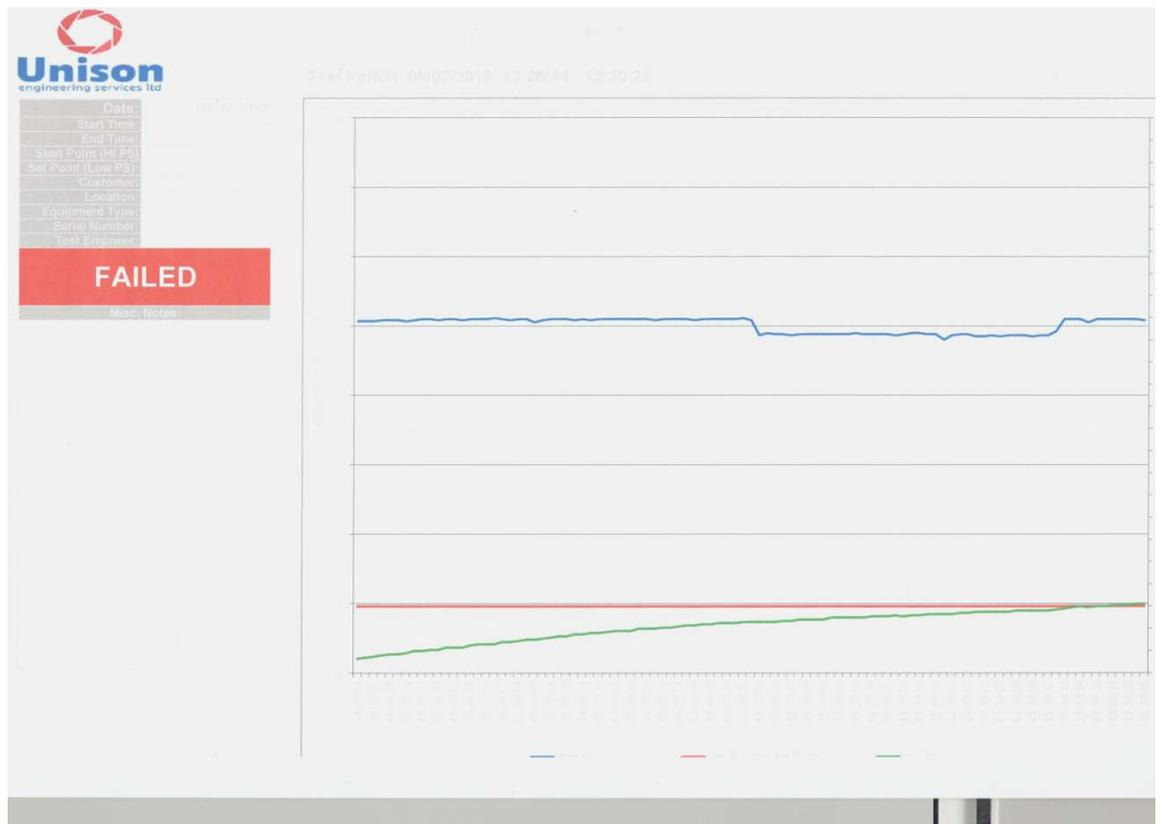
Leaking plate fitted. Pressure difference 5.07 bar, set point 60 mbar. Blue line high pressure side pressure, red line low pressure side set point, green line low pressure side pressure.
