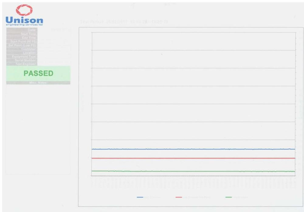
Leaking plate fitted. Pressure difference 1.471 bar, set point 60 mbar. Blue line high pressure side pressure, red line low pressure side set point, green line low pressure side pressure. At this low pressure difference no leak detected.
