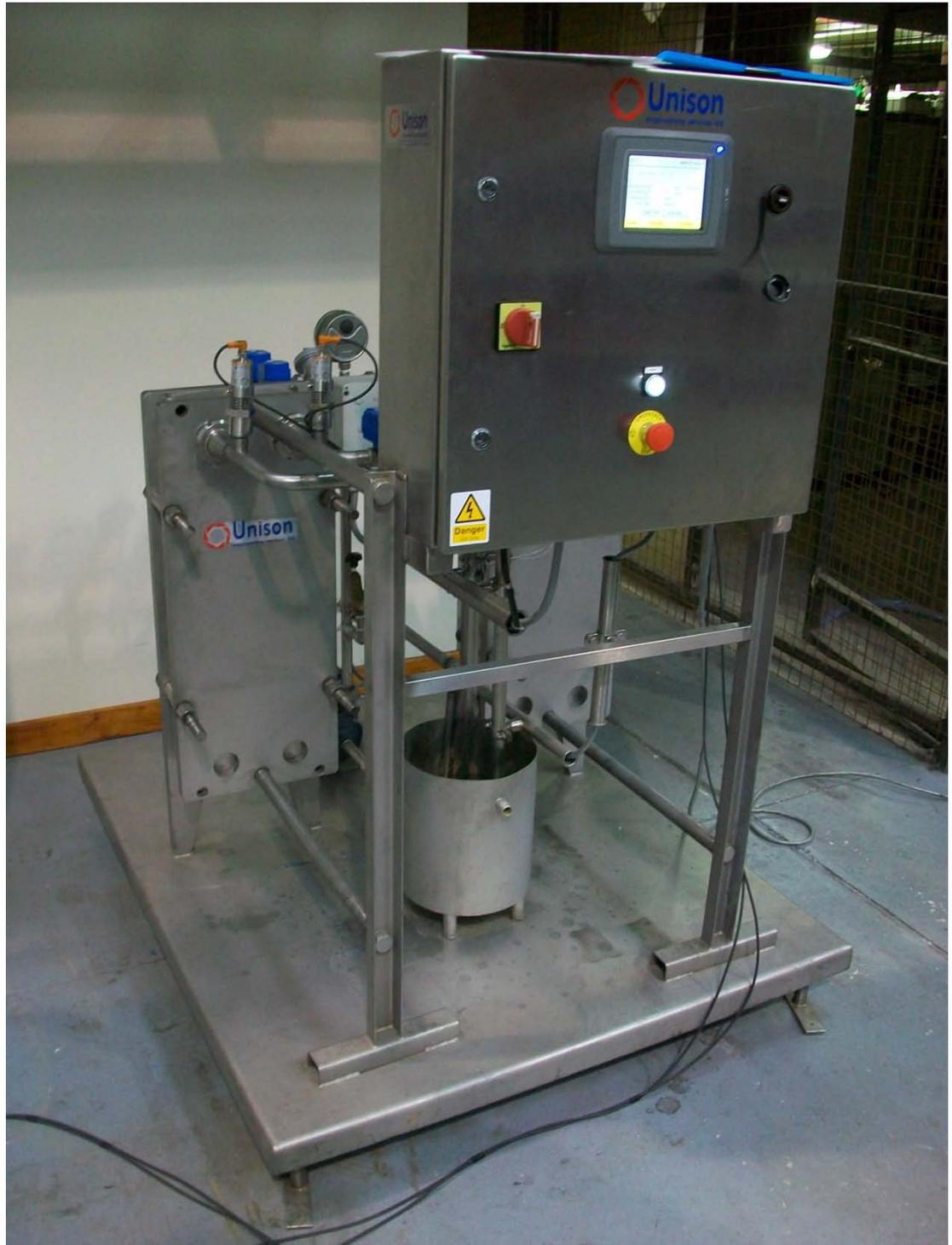
The test unit at Unison. The small vessel bottom middle enabled recycling around the high pressure side. There are two plate heat exchanger units although only one was required for these tests.
