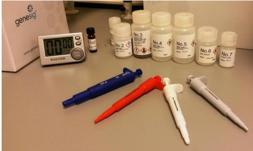
**Figure 1:** DNA extraction buffers and colour-coded pipettes from the genesig® Lab-In-A-Box.
