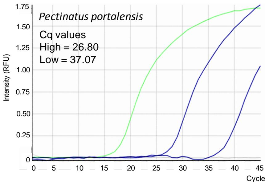
**Figure 4:** Detailed view of the DNA amplification curves of two concentrations of *Pectinatus portalensis*. The positive control (green), the high concentration (blue, leftmost) and the low concentration (blue, rightmost) samples are shown, along with their corresponding Cq values.
