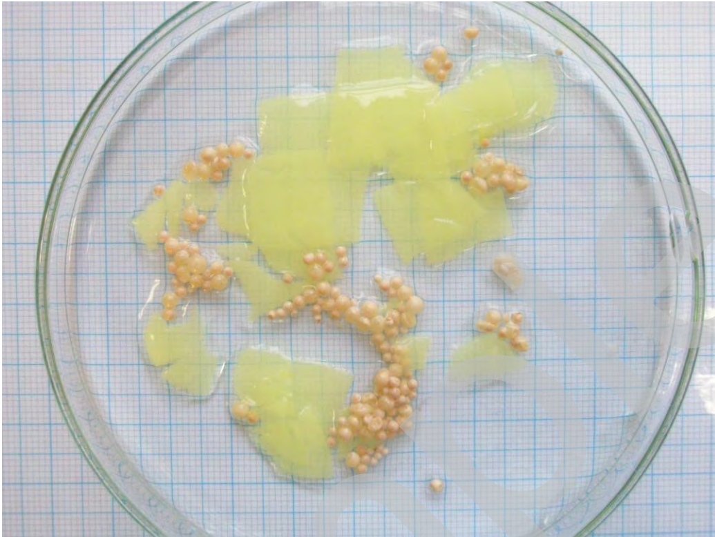
PLATE 2 Shows the remains of the capsule on a glass Petri dish (top) and the variable sizes and shapes of the spansules (bottom), both photographed against a millimetre-squared background
