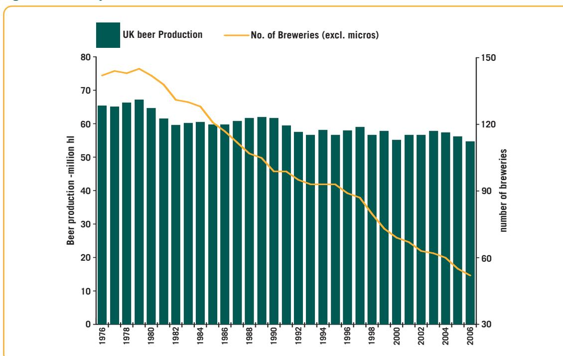
There has been a steady growth in the market share of lager to the point where it exceeded the volume of ale production in 1990. The lower fermentation temperature and cold conditioning period required for lager production results in a higher refrigeration demand and consequent greater electricity consumption. Lager now accounts for over 70% of UK beer sales.
