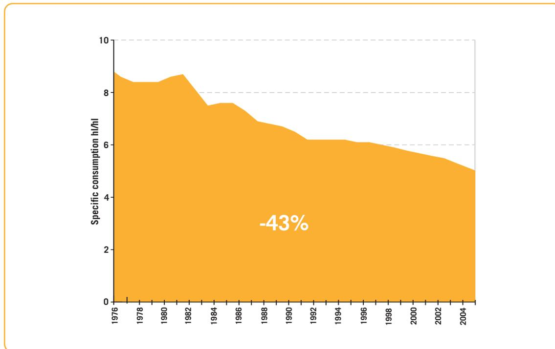
It has been demonstrated that water and energy efficiencies go hand in hand. Reduced volumes mean less pumping demand and lower heating and cooling loads.
